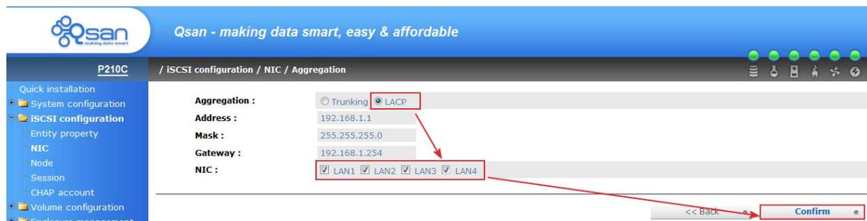
2. Add a LACP Group on the gigabit switch. Set port 1, 2, 3, 4 as activite. These four ports are mapped to the iSCSI data port of **P210C**.
