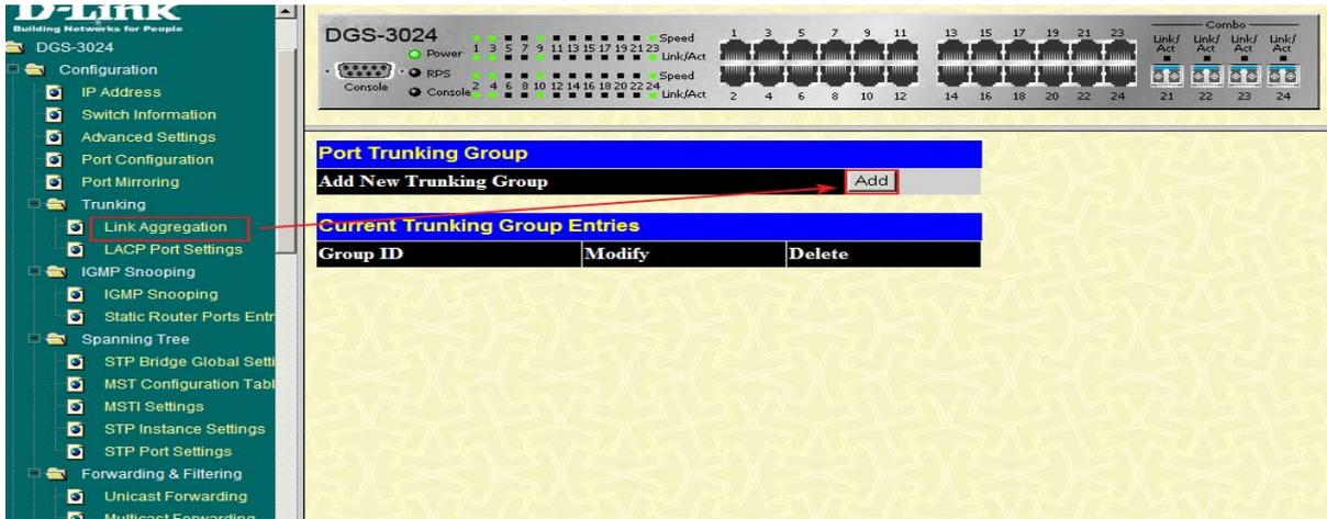
3. Select port 1, 2, 3, 4, and then press “Apply”. These four ports are aggregated to a group and are mapped to the iSCSI data port of **P210C**.
