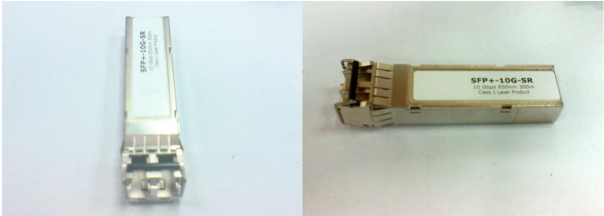
Figure 2, SFP+ -SR transceiver
