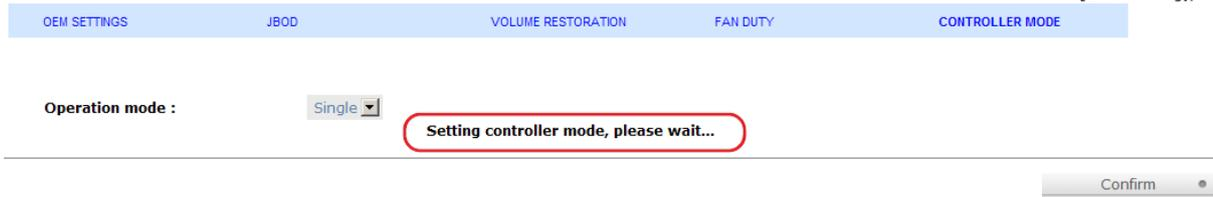
4. It is necessary to shutdown the subsystem to make new setting take effect when switching the operation mode.
