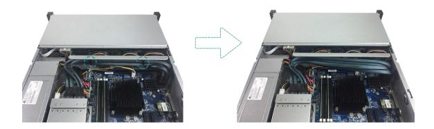
2 Hold both ends of the fan module and lift it upwards to remove it.
