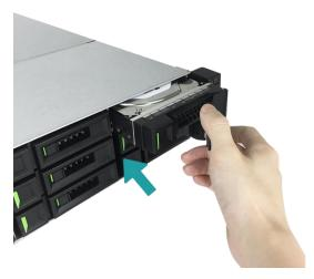
2 Push the disk drive lock from right to left to lock the drive tray.
