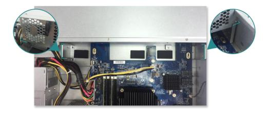
3 Push the fan module all the way down and put the cable back into the cable holder.
