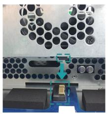
② Slide the fan module into the fan holder rail. Make sure both sides are aligned properly as illustrated below.
