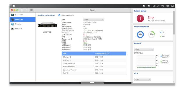
If you see the error message shown above, which means your PSU has encountered an issue and need to be replaced immediately. To replace the malfunction PSU, please refer to <a href="mailto:chapter 3.5 Replace Malfunctioning PSU">chapter 3.5 Replace Malfunctioning PSU</a>. After the new PSU is successfully installed, the PSU status LED will be green and you can see the PSU status displaying "Good" on QSM.
