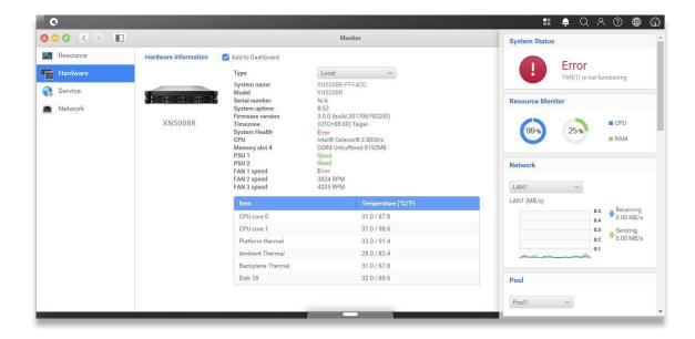
If you see the error message shown above, which means your fan module needed to be replaced immediately. To replace the malfunction fan module, please refer to <u>chapter 3.4</u>
