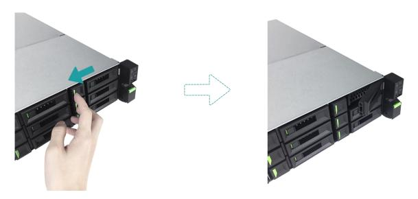
(2) Hold the carrier handle and pull out the disk drive tray, repeat the steps above to remove other disk drive trays.
