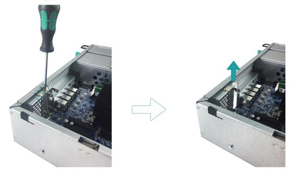
3 Align the card's connector with the expansion slot, and insert the card into the slot.
