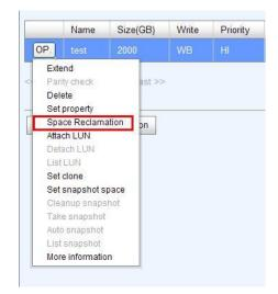
This function will check the whole data of the VD which allocated on the RAID sets in background, see if there are any spaces could be reclaimed.
