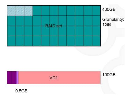
Even only 2.5 GB of data was written into the VD, there is still 3GB of physical space on the RG allocated to the VD.
