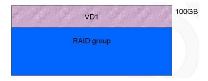
The storage will tell the server (host) that there is a 100GB VD1 can be used, and pretending the 100GB VD1 has been allocated on the RG. But in fact, the spaces on the RG will not decrease until reading or until any data is really written into the VD1 from the server (host). Such as the below illustration, there is a VD created on a thin provisioned RG, but the Free space will not be used before writing any data into the VD.
