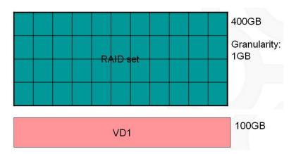
The RAID set will be divided by the Granularity (1 GB) which is the minimum size while allocating the space to a VD.
