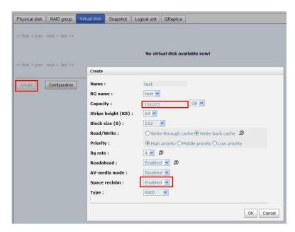
Enabling this option means when the data is written into the VD, the system will check in real time if there is space could be reclaimed.
