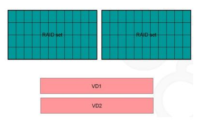
The system has its own policies (the health status of the RAID sets, the available capacity of the RAID and etc.) to judge which one of the RAID sets is proper to be allocated to a VD while space is demanded as the data changes. And you may observe which one of the RAID sets had been allocated with the data from the RG page on the web GUI when you clicked on the RG. For example, please see the below illustration, the space on the RAID set 2 is allocated more than on the RAID set 1.
