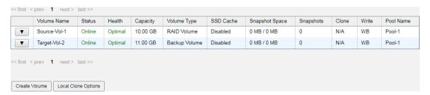
Figure 12-15 List Source and Target Volumes for Local Clone
