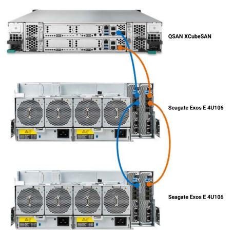
Figure 2 One XCubeSAN / Two Seagate Exos E 4U106 / Dual Path
