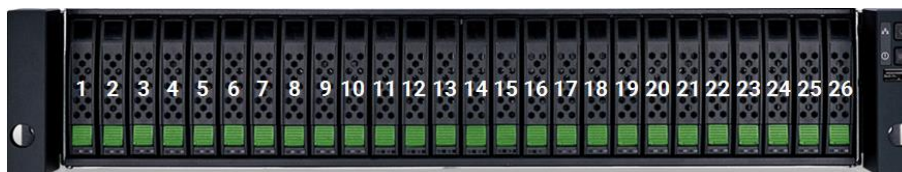
Figure 2-4 System Disk Drive Numbering for the XCubeSAN Series
